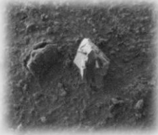
Scanning Electron Microscope Images of Possible Micrometeorite Impacts on Aerogel
