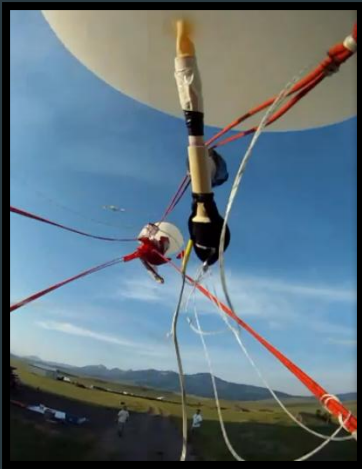
Early Helium vent test for neutral buoyancy valve
